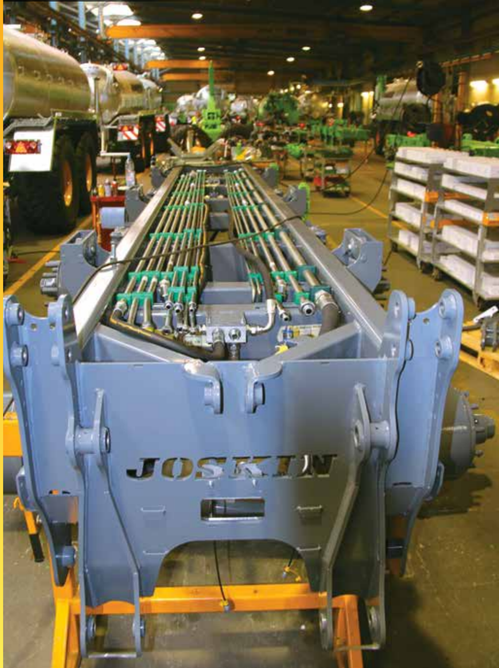
A Euroliner chassis is fitted out before the tank goes on
