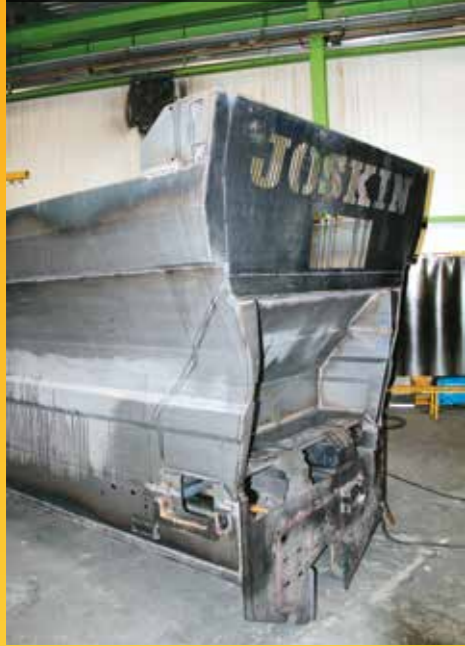
A Tornado 3 muck spreader before painting
